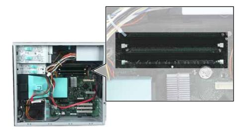
**4** If you are removing a DIMM from the memory module bank, gently pull the plastic tabs away from the sides of the memory module and remove it.
